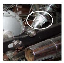
riding on rough roads. Place the motorcycle on it's stand and turn the adjustment ring to change the setting.
